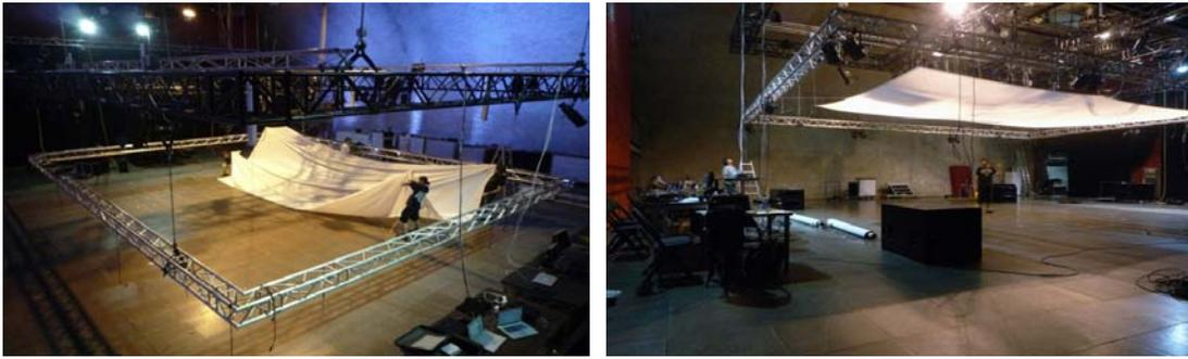
Figure 2. The projection setup of the event consists of four projectors projecting onto a movable, fabric projection surface mounted horizontally on electronically controlled actuators.
