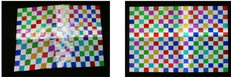
Figure 9. Displaying a checkered pattern on four overlapping projections using a non-planar projection surface leads to visual problems like nonlinear transformations and overlapping artifacts (left). The corrected result (right) shows none of these problems at all, with the exception of variations in brightness because of overlapping projections.
