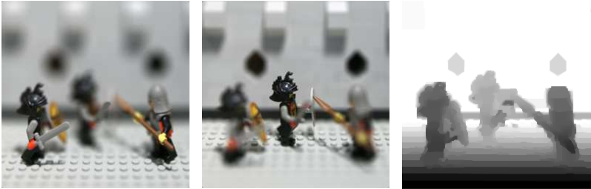
Figure 6. (Left and center) Subset of images from the focal stack obtained with our algorithm. (Right) 3D reconstruction image where depth is presented as a grey color. The size of the plenoptic image is n=512 and m=17 .
