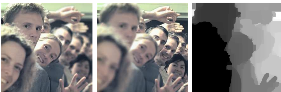
Figure 4. (Left and center) Subset of images from the focal stack obtained with our algorithm. (Right) 3D reconstruction image where depth is presented as a grey color. The size of the plenoptic image is n=291 and m=9 .
