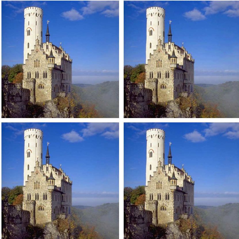
Figure 2. Original (top left), encoded with PVRTC (up right), encoded with squish (bottom left) and with line matching (bottom right).
