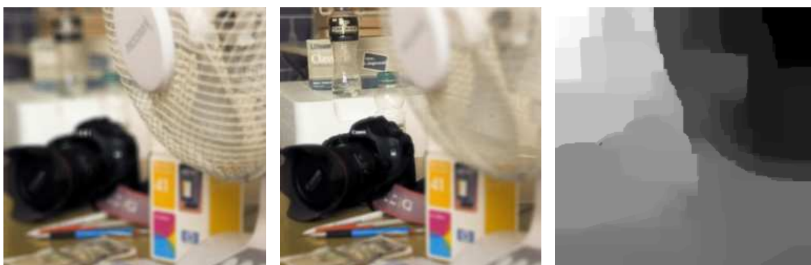
Figure 5. (Left and center) Subset of images from the focal stack obtained with our algorithm. (Right) 3D reconstruction image where depth is presented as a grey color. The size of the plenoptic image is n=249 and m=9 .
