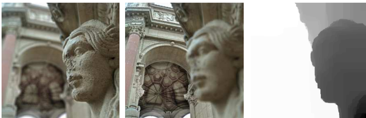
Figure 3. (Left and center) Subset of images from the focal stack obtained with our algorithm. (Right) 3D reconstruction image where depth is presented as a grey color. The size of the plenoptic image is n=291 and m=11 .
