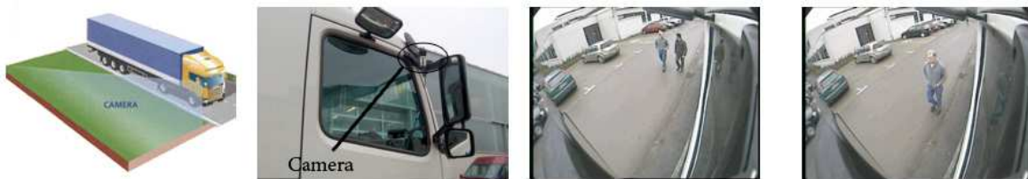
Figure 1. (a) Blind spot of a truck. (b) Blind spot camera mounted on truck. (c) And (d) are test frames of the blind spot camera.
