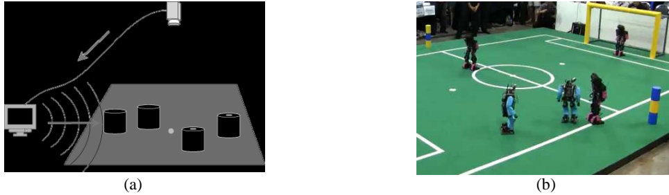
Figure 1. (a) Global vision system, Small Size league. (b) Local Vision of Humanoid league
