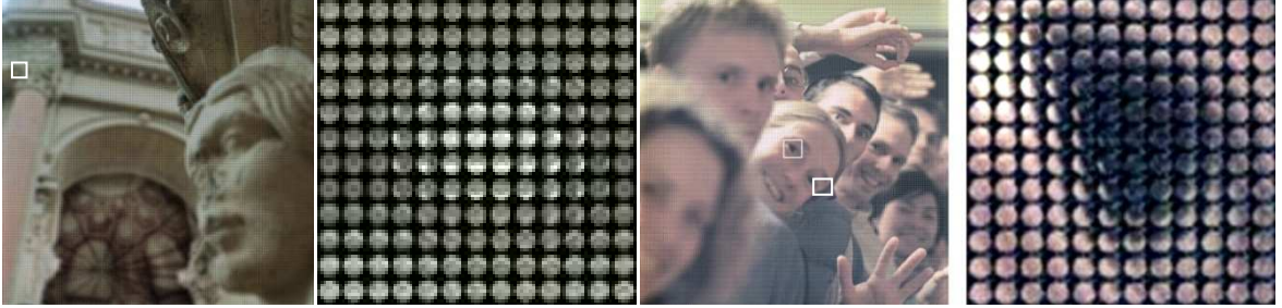
Figure 2. Plenoptic images and details from the white square in the plenoptic images [4].
