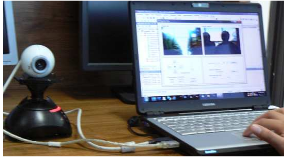
Figure 1. The main components of the tracking system (webcam, polar motion stage, and PC)
