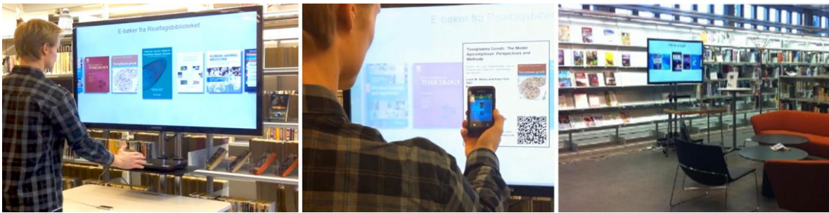
Figure 3. Browsing gesture while searching for e-books. When an e-book is selected, the QR code is scanned and the link to the e-book sent to the user's email address. Placement of the system within the library (Okun et al., 2013).
