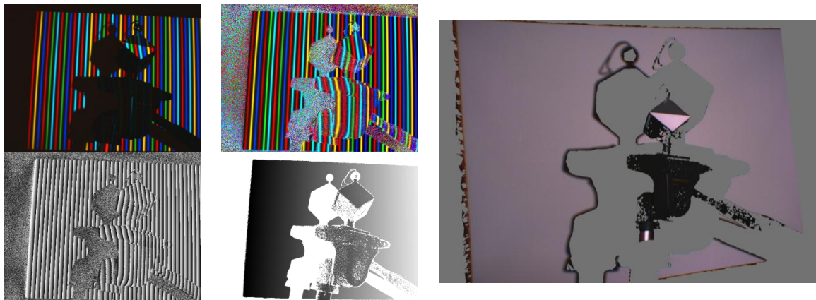
Figure 5. The SpyderCUBE™ on a tripod. Top-left is the input image (1/12), top-middle is equalized image (1/12), bottom-left is wrapped phase, bottom-middle is unwrapped phase, and right is 3D reconstruction
