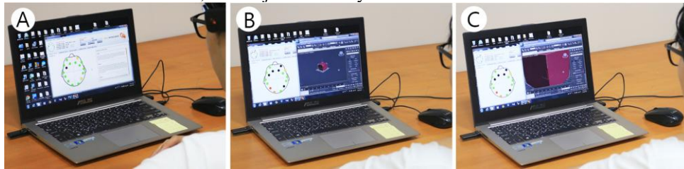
Figure 2. Scenario demonstration: A) user wears EPOC+, and check the electrode contact quality; B) the user started to use imagination command to zoom out the box of the viewport; C) the user smoothly zoom in the box of the viewport.
