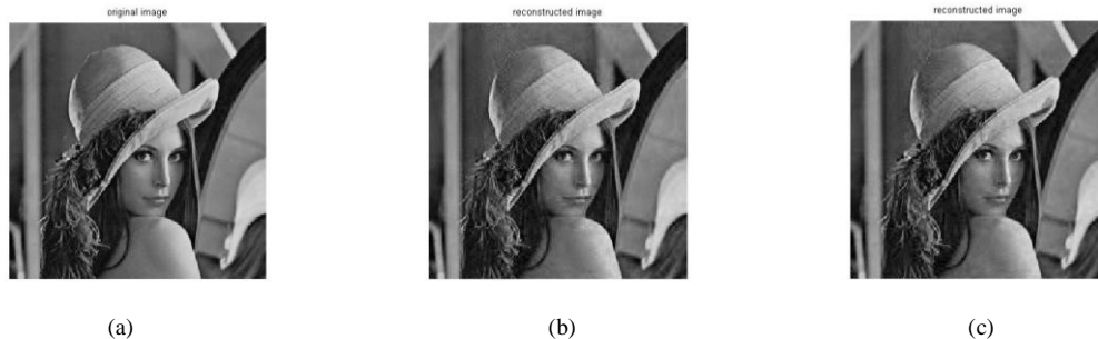
Figure 2. Subsampling rate \alpha = 0.8 , taking wavelet transform matrix as \Psi : (a) Original image. (b) Taking Gaussian random matrix as \Phi . (c) Taking Bernoulli matrix as \Phi
