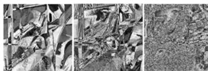
Figure 6. Results of encrypted image by using three other bit-pairs of host image: left, middle and right image is the result of respectively 7-6, 5-4 and 3-2 bits
