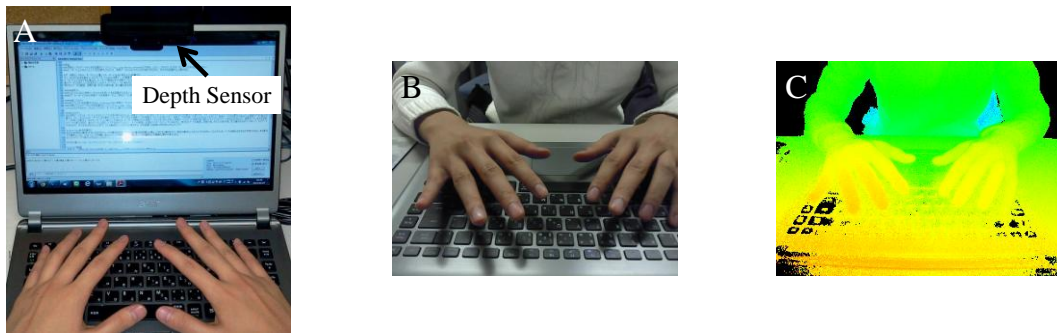
Figure 1. Setting of a depth sensor (A). Color image (B) and the depth map (C) imaged by the depth sensor.
