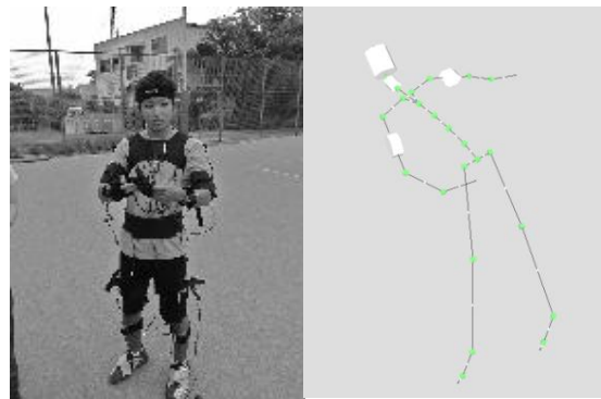
Figure 1. Motion Capturing System and captured body parts (MVN)
