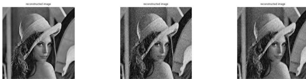
Figure 3. Subsampling rate \alpha = 0.8 , taking Gaussian random matrix as \Phi : (a) Taking Daubechies10 wavelet matrix as \Psi . (b) Taking DCT matrix as \Psi . (c) Taking Fourier matrix as \Psi
